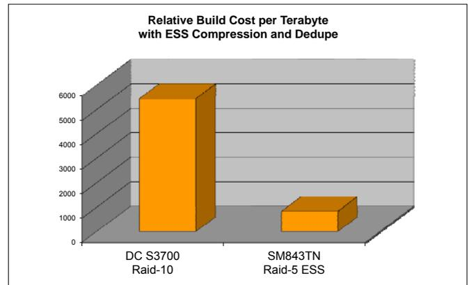
While enhanced ESS cuts manufacturing costs per terabyte even further, it also improves media life by reducing the amount of data written to the media either through compression or the virtualization of deduplication. Accordingly, a 2x increase in logical space utilization decreases total wear by a factor of two, while increasing the number of supportable daily overwrites by a factor of two.
