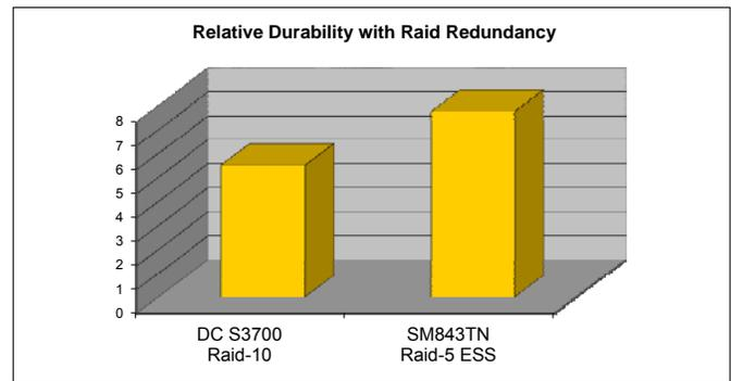
24 S3700 SSDs, managed by Linux Raid-5 will only write 40,000 IOPS – too slow for practical use in all-Flash devices. The same media, managed by Linux Raid-10, will deliver 444,000 write IOPS. But the ESS managed Raid-5 set of 24v SSDs will deliver far in excess of a million write IOPS.
