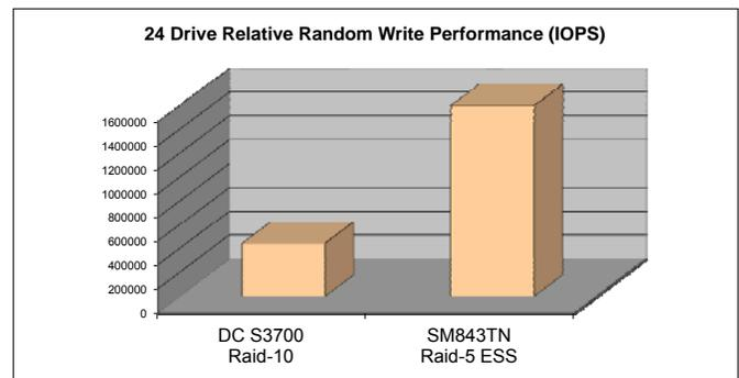
But what is most compelling, as the following table shows, is that while ESS delivers more durability in terms of total writes per day as well as radically greater random write speed, ESS delivers these capabilities in our basic
